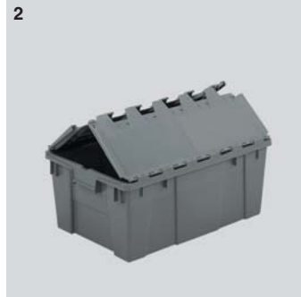
2 40 litres - Ref. 1BK40** inter-stacks with refs. 1BK52 & 1BK62 Ext. dim.: L 600 x w 400 x h 250mm Ext. dim.: L 23.6 x w 15.7 x h 9.8" Int. dim.: L 501 x w 328 x h 205mm Int. dim.: L 19.7 x w 12.9 x h 8.1" Nested height: 67mm/2.6" Weight: 2.9 Kg/6.4 lbs. Colour: light grey
