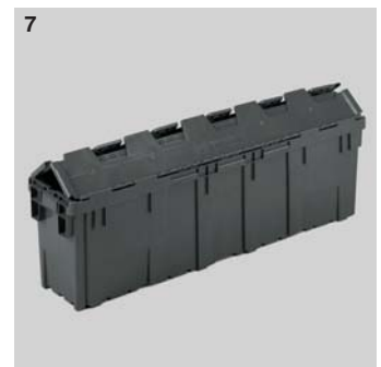
7 78 litres – Ref. 1B561 with drainage holes in base Ext. dim.: L 1,216 x w 280 x h 365mm Ext. dim.: L 47.9 x w 11.0 x h 14.4" Int. dim.: L 1,121 x w 206 x h 308mm Int. dim.: L 44.1 x w 8.1 x h 12.1" Nested height: 115mm/4.5" Weight: 6.2 Kg/13.6 lbs. Colour: dark grey
