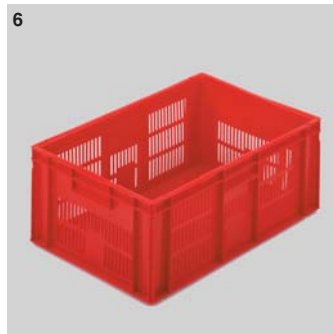
6 45 litres - Ref. 2A046 polypropylene solid base, ventilated sides, incorporates strapping facility for secure palletisation. Ext. dim.: L 600 X w 400 X h 235 mm Ext. dim.: L 23.6 X w 15.8 X h 9.3" Int. dim.: L 555 X w 355 X h 220 mm Int. dim.: L 21.9 X w 14.0 X h 8.7" Wt: 1.88 kg/4.1 lbs., Colour: red. SKU quantity: 20
